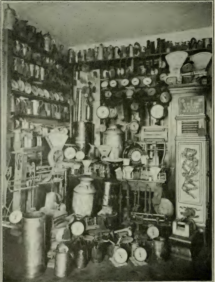
FIG. 229. Numerous designs of faulty weighing and measuring equipment taken out of service by Weights and Measures officials and later on destroyed.
